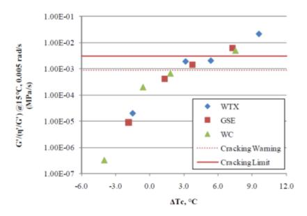
Figure 12: Glover viscosity function vs.  $\Delta Tc$  (note Glover viscosity function and Glover-Rowe parameter give the same information – one is just a simplified version of the other)
