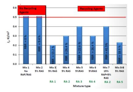
Figure 2: J<sub>c</sub> computed from SCB test at 25°C
