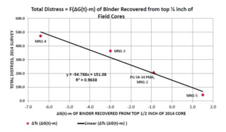
Figure 6:  $\Delta$ Tc from binder extracted from field cores versus total distress
