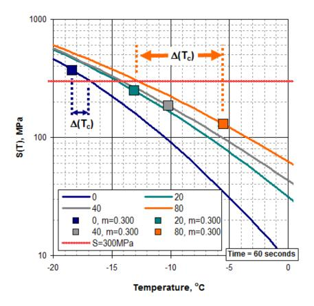
Figure 11: S(T) (t=60 seconds) for GSE binder showing determination of  $\Delta Tc$  (after Anderson et al., 2011)
