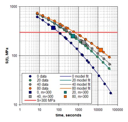
Figure 10: BBR master curve for binder data sets illustrating S(60)=300 MPa and m-value = 0.300 (after Anderson et al., 2011)
