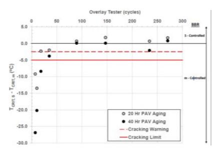
Figure 9:  $\Delta$ Tc versus overlay tester results
